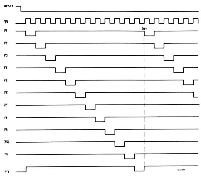
Note: The matrix scanning starts (after the power on reset) at the second arrival in output of F1 (\*) from B1 to B6 i continuous sequence.
