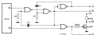
The antibounce time can be regulated by acting on constants R1-C1 (antibounce on pressing a key) and R2-C2 (antibounce on release of key). In the application diagram of the device an antibounce of 18 ms is established C1 = C2 = 18 nF and R1 = R2 = 1  $M\Omega$ . The time constants must not however be 12 ms.
