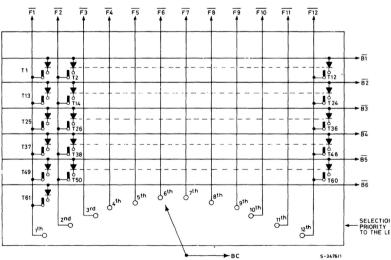
If the device is used with selection of the first key to the left connect the control bar BC to  $V_{SS}$ . For different priorities of the first key to the left connect BC to the selection frequency for the selected priority key. In this case BC must have a pull-up of 5.6  $K\Omega$ .
