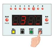
To exit the PROGRAMMING mode, press the **PROG** button: in this way the time appearing on the display will be saved in the memory with the number indicated by the lighting up of one of the **8 red LEDs** (for example, if upon exiting PROGRAMMING mode the LED number 6 is on, the time just programmed will be saved in the memory as Time number 6).
