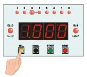
Once you have reached time number 8, by pressing the button again, you start again from time number 1 and so on. The time currently shown on the display and indicated by the corresponding **red LED** lighting up, will be the one used by the Timer at start-up (in the example on the right, Time number 4 has been selected).
