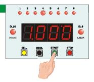
During the countdown, the **red LED "LAMP"** is on, indicating that the enlarger lamp is activated.
