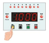
Once the desired Time to be programmed has been selected, press the **PROG** button to enter the PROGRAMMING mode.
