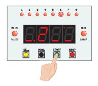
O Button  $\triangle$  (*STOP*) - Each press inserts a value from 0 to 9 to the selected digit. Once the value 9 has been reached, pressing the button again restarts from the value 0 and so on.
