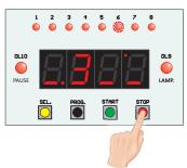
To exit the PROGRAMMING mode, press the **PROG. MEM.** button: in this way the time appearing on the display will be saved in the memory with the number indicated by the lighting up of one of the **8** red LEDs (for example, if upon exiting PROGRAMMING mode the LED number 6 is on, the time just programmed will be saved in the memory as Time number 6).
