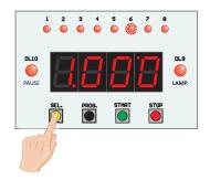
Once the desired Time to be programmed has been selected, press the **PROG. MEM.** button to enter the PROGRAMMING mode.
