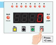
When the PEDAL socket is programmed as **FOCUS**, each pressure of the pedal (or of any other actuator connected to the socket) turns on the enlarger lamp without timing.
