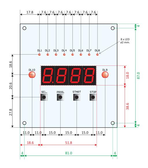
Board Dimensions (Dimensioni scheda): **89 x 95 mm**. DL10 (LED "PAUSE") and DL9 (LED "LOAD"): Ø**3** or Ø**5 mm**. DL1-DL8 (Selected Time - Tempo Selezionato): Ø**2 mm**.
