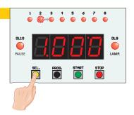
Each time the button is pressed, ONE of the 8 times programmed by the user will be shown on the display (the corresponding number will be indicated by ONE of the 8 red LEDs).
