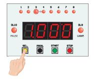
Once you have reached time number 8, by pressing the button again, you start again from time number 1 and so on. The time currently shown on the display and indicated by the corresponding red LED lighting up, will be the one used by the Timer at start-up (in the example on the right, Time number 4 has been selected).
