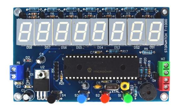
T-1000 DIGITAL STOPWATCH H:MM:SS.ddd based on PIC16F887 with 7 SEGMENT DISPLAY
