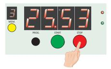
In this situation, by pressing the **START** button, the Timer restarts from where it was interrupted, while by pressing the **STOP** button once again, the counting stops definitively (FINISH) and the Timer is ready to be started again by the user (green "**READY**" light on).
