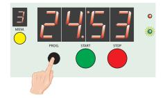
During programming the Time, ONLY one digit lights up on the display at a time (i.e. the one selected for entering the value to be programmed): the remaining digits on the display are "hidden" and their positions are indicated by **underscores**.
