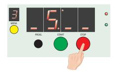
To exit the **PROGRAMMING**, press a second time the **PROG** button: in this way, the time appearing on the display will be saved in the memory with the number indicated by the small display at the left: for example, if upon exiting PROGRAMMING mode the value shown by small display is 3, the time programmed will be saved in the memory as **Time number 3**.
